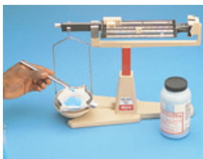
Figure 6 On this type of mechanical balance, the sample is balanced by moving masses on several beams.
