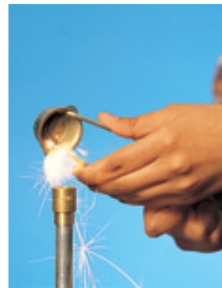
Figure 3 To generate a spark with a striker, pull the side of the handle containing the flint up and across.
