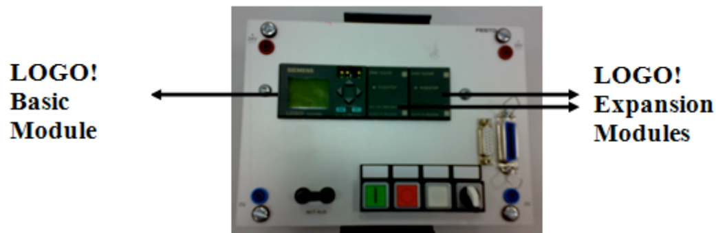
Figure 2.9: LOGO! Basic & Expansion Modules on Edutrainer Compact
