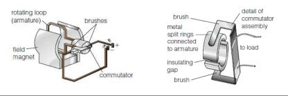
Electric Generator: a device that converts mechanical energy into electric energy.
