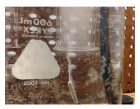
J HOOKS ARE PLACED ON THE **OUTSIDE** OF THE TEST TUBE, AND IN THE NOTCH IN THE TEST TUBE HOLDERS, AS SHOWN ABOVE LEFT AND RIGHT.
