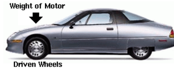
Figure 7: Front Wheel Drive weight distribution
