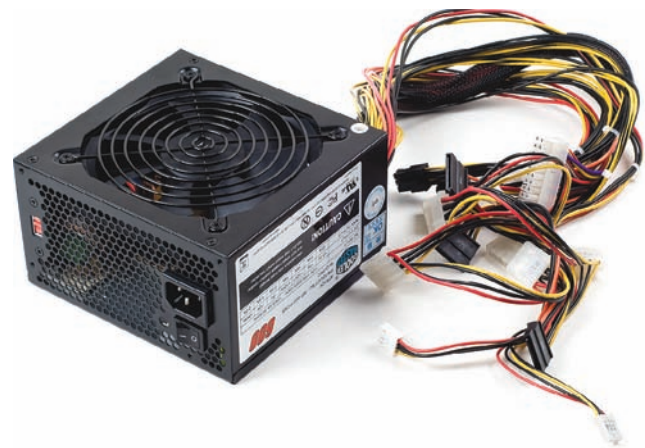
• Figure 3.41 Power supply
