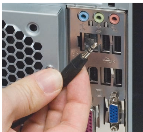
• Figure 3.17 Mini-audio jacks and plug
