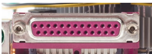
• Figure 3.29 Parallel port
