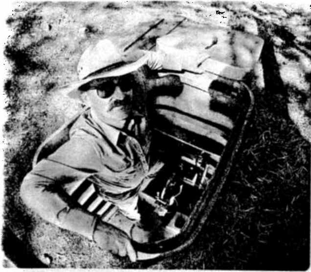
GEOLOGY A creepmeter monitors creep, the downslope movement of soil.
