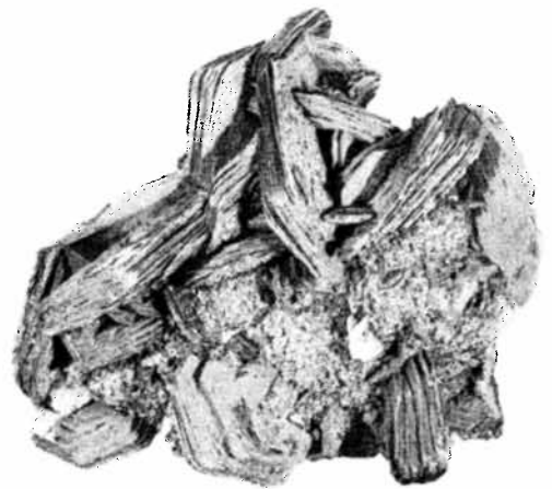
CLEAVAGE TEST Mica splits well in only one direction.
