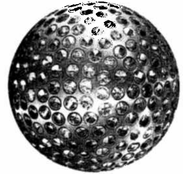
SATELLITE LASER RANGING A satellite covered with reflectors is used to measure plate movement.
