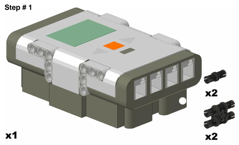
Attach the connect four pieces and the friction pin into the NXT as shown.
