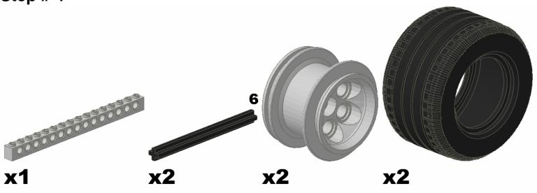
Attach the wheels and the tires with the six stud axles. Clip on the wheel assembly as shown. Place pins into the ends and two holes in from the ends of the 15 stud beam and place it across the motors as shown.
