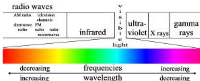
Different colors on the electromagnetic spectrum have different wavelengths (nanometers) and different frequencies (hertz).
