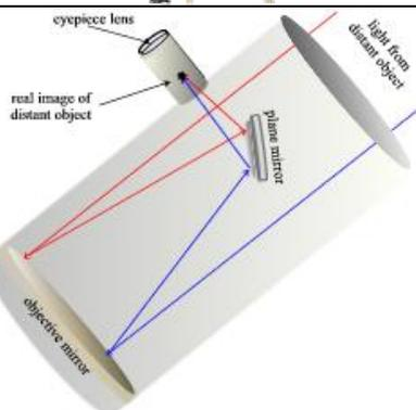
**reflecting telescope (Figure 3.41B p. 222)**
