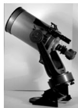
The lens in a refracting telescope and the mirror in a reflecting telescope collect as much light as possible from distant objects. These collectors then focus the light into an image. The further away the image is from the lens, or the mirror, the greater the magnification. For the greatest magnification the telescope needs to have as large a distance as possible between the object being viewed and its image.
