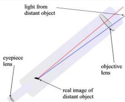
**refracting telescope (Figure 3.41A p. 221)**
