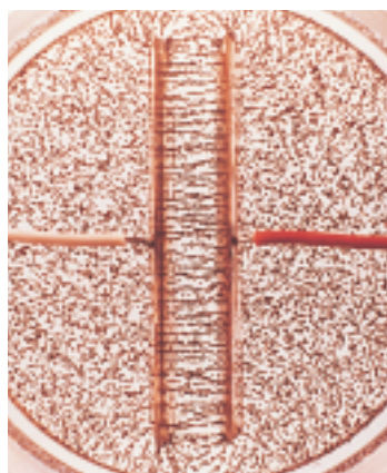
FIGURE 21–8 A representation of an electric field between parallel plates is shown.
