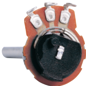
FIGURE 22–7 An inside view of a potentiometer shows the coils and the sliding contact wire.
