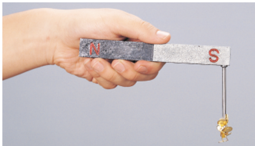
FIGURE 24-3 If you touch an iron nail with a magnet, the nail will become magnetized and will in turn attract other iron objects. However, as soon as the magnet is removed, the nail will lose its magnetism.
