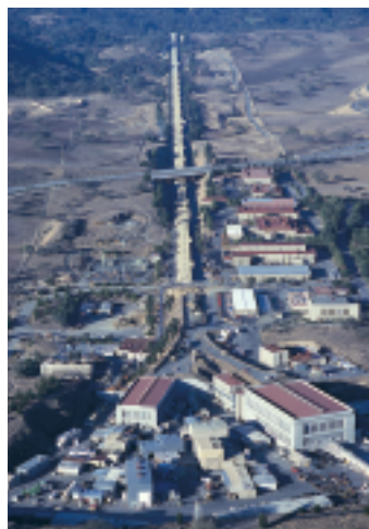
FIGURE 30–7 The linear accelerator at Stanford University is 3.3 km long (a) . Protons are accelerated by changing the charge on the tubes as the protons move (b) . (Not drawn to scale.)
