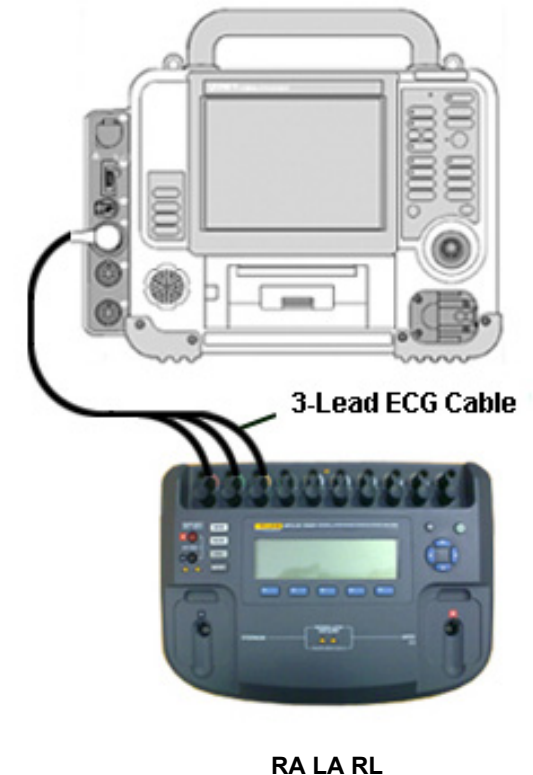
Figure 5.37—ECG 3-wire connection
