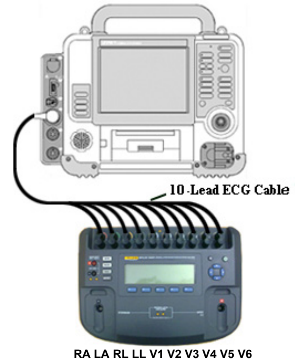
Figure 5.33—ECG lead connections
