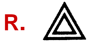
R. Emergency Flashers
