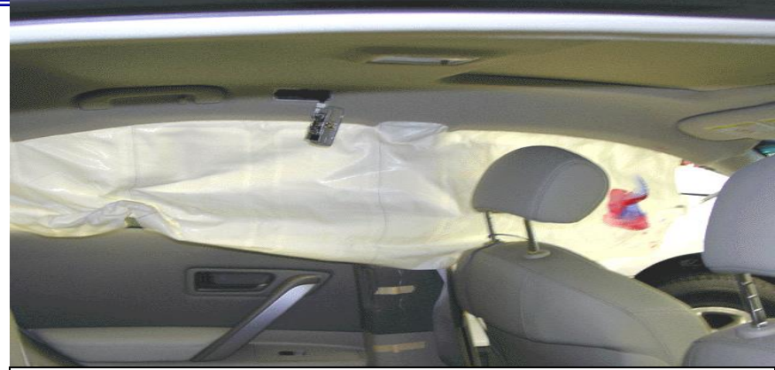
Side air bag deploys in crash test. Red area shows where the dummy's head impacted the airbag.
