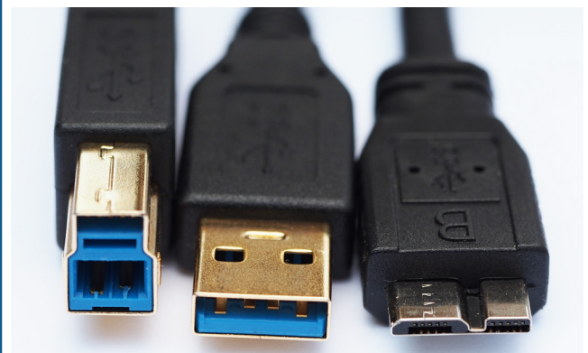
USB 3.0 Standard-B Plug USB 3.0 Standard-A Plug USB 3.0 Micro-B Plug
