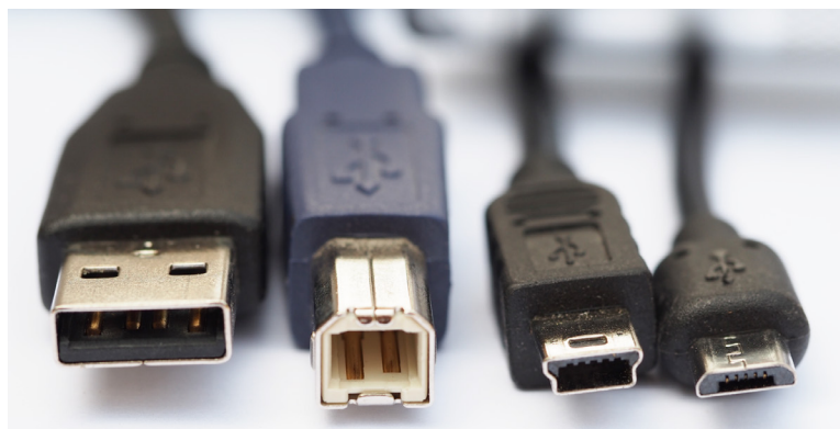
USB 1.0/2.0 Standard-A Plug USB 1.0/2.0 Standard-B Plug USB 1.0/2.0 Mini-B Plug USB 1.0/2.0 Micro-B Plug
