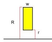
The washer is formed by revolving a rectangle about an axis
