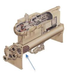
10. A chiller evaporator consists of refrigerant lines enclosed in a <u>shell</u>. Water circulates in the shell, around the refrigerant lines.
