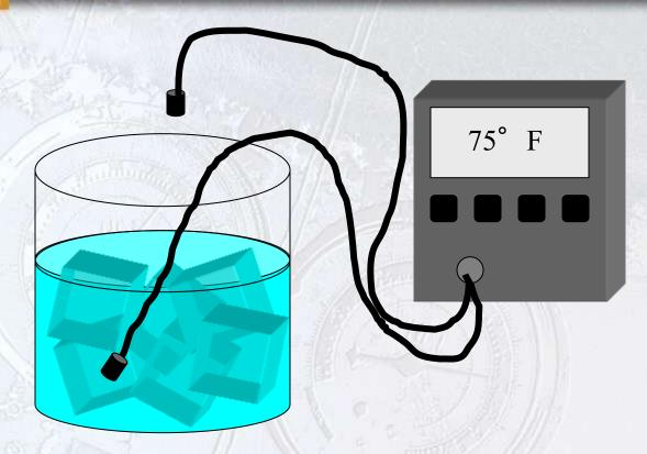
The probe of the thermometer should be submerged in the liquid if possible
