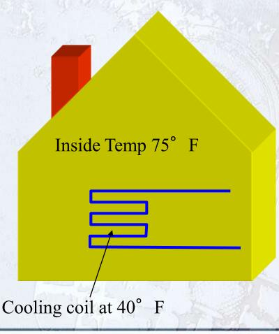
Heat flows naturally from the air inside the house to the cooling coil (evaporator)
