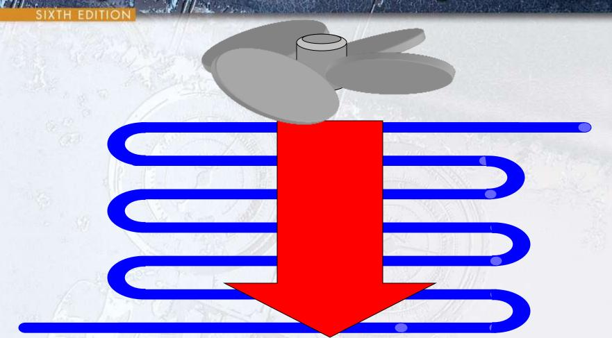
FORCED DRAFT EVAPORATOR PUSHES AIR THROUGH THE COIL
