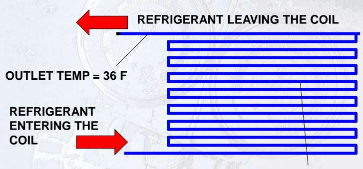
**EVAPORATOR SATURATION TEMPERATURE = 25 F**
