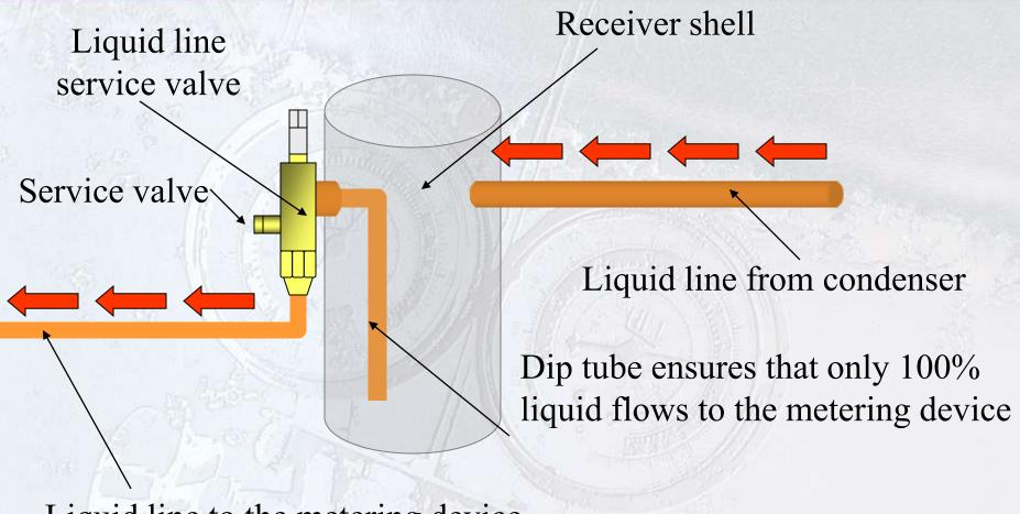
Liquid line to the metering device
