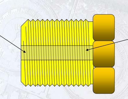
Hole is filled with a low temperature solder
