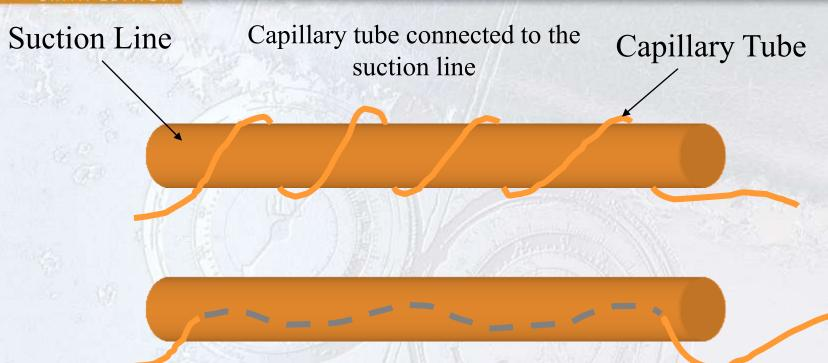
Capillary tube run inside the suction line
