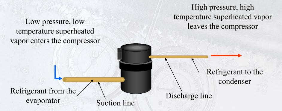
Refrigerant in the compressor is superheated, so it does not follow a pressure/temperature relationship!
