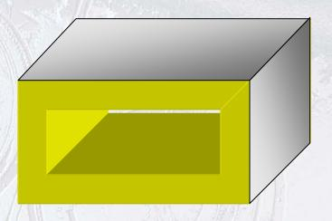
Notches are cut in the board to facilitate the folding of the board into a duct section
