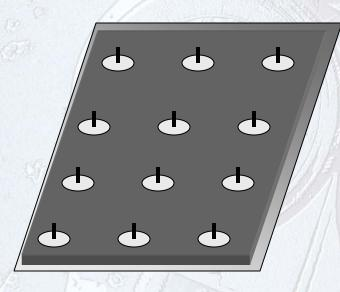
Inulation liner is glued in place on the duct and pierced by the tabs
