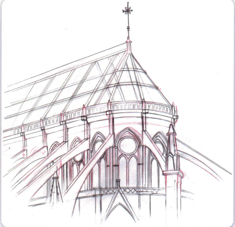
Figure 1-26: The skeleton construction of Gothic architecture.
