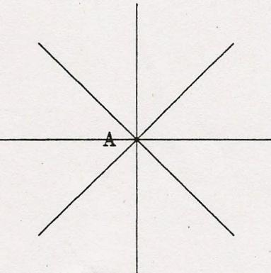
Draw 8-1" lines radiating uniformly from point A using the polar coordinate system.
