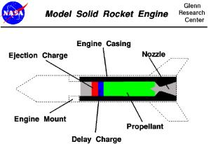
The rocket engines use in our model rockets work by igniting a solid fuel, creating super heated gasses that escape through the clay nozzle at the base. The force of this gas escaping is enough to lift the rocket off the ground.
