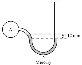
If the pressure of the gas labeled A is 1 atm, what is the atmospheric pressure?
