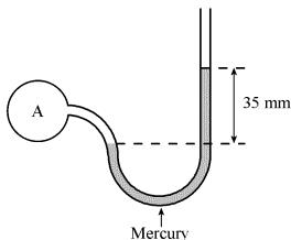
If the atmospheric pressure is 730 torr, what is the pressure of the gas labeled A?
