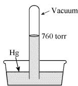
In the image above, if the mercury were replaced by water and the atmospheric pressure remained the same, (assuming the column is tall enough to contain it,) what height would the water reach?
