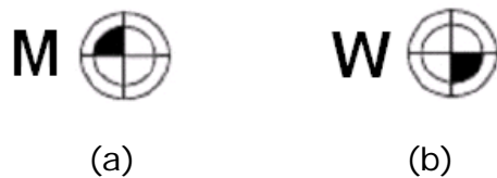
Fig. 1.7: (a) Left: "M" Machine zero point symbol. (b)Right: "W" Workpiece zero point symbol.
