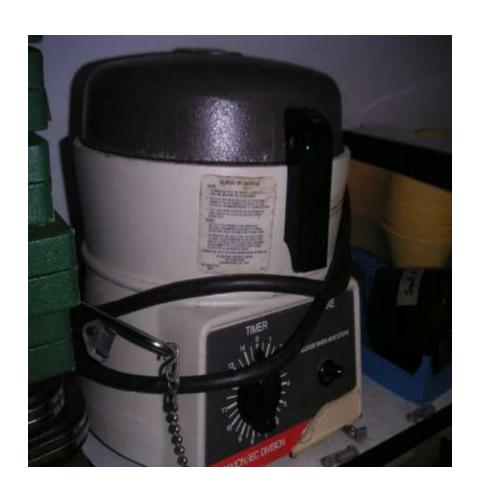
An instrument used to determine the ratio of packed red blood cell volume to whole blood volume.
