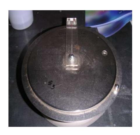
Small instrument used to read capillary tubes.
