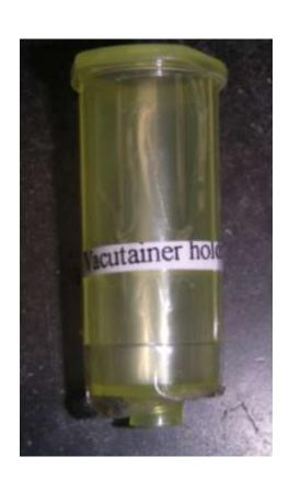
Vacutainer, cylinder shaped, holder that accepts a vacutainer tube and needle.
