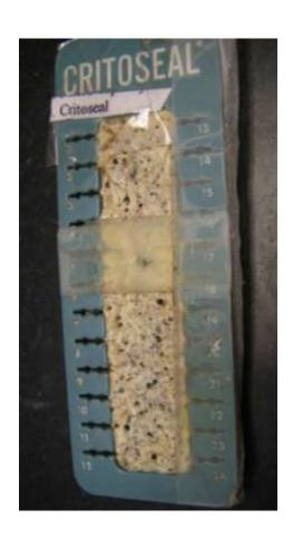
Seals capillary tubes without heat and very quickly.
