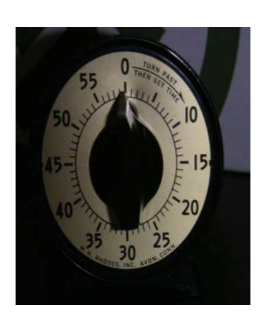
Device used to accurately time periods for when samples must be rotated or otherwise.
