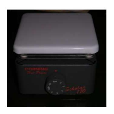
Equipment used to heat solutions without an open flame.
