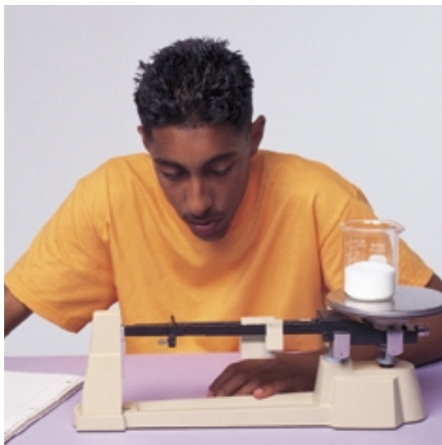
The mass of the table salt and beaker together is 230 g. Therefore, the mass of the salt is 70 g.
