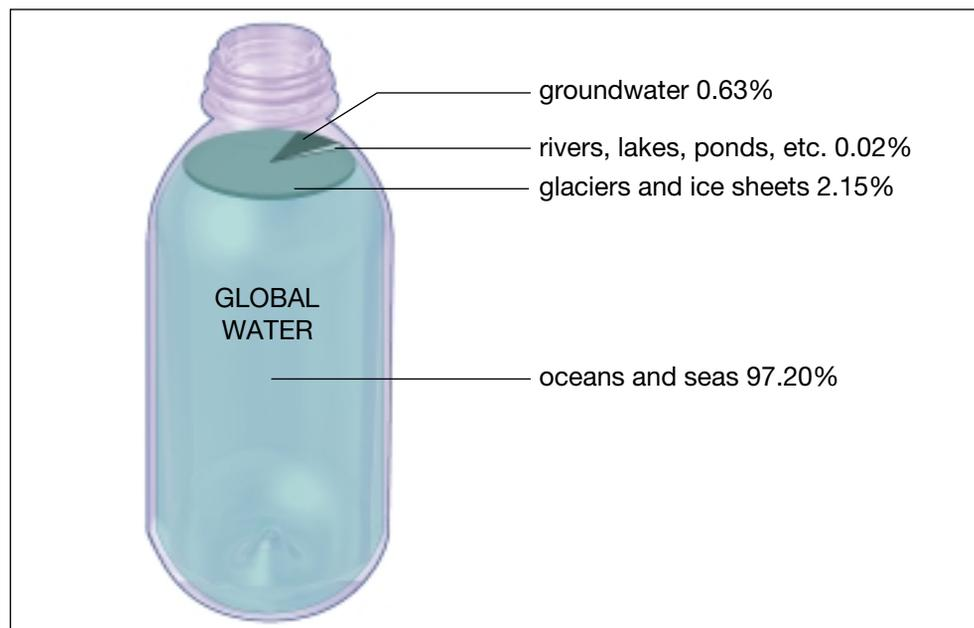
**Figure 5.3** This "bottle graph" shows the distribution of water on Earth, by volume.
