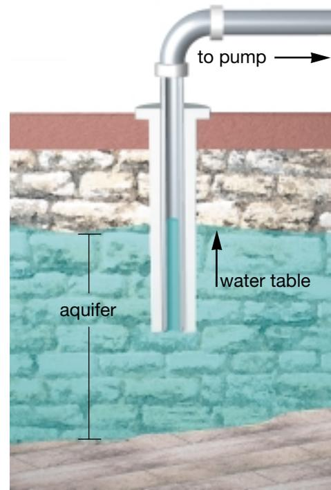
Figure 5.47 Wells are dug deep enough to reach a point below the water table.
