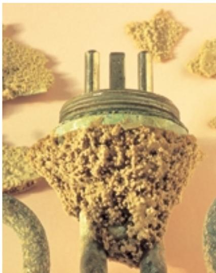
**Figure 5.85** This electric kettle element shows deposits of salts left by water evaporation.
