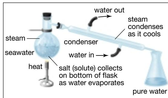
**Figure 5.96B** The process of distillation
