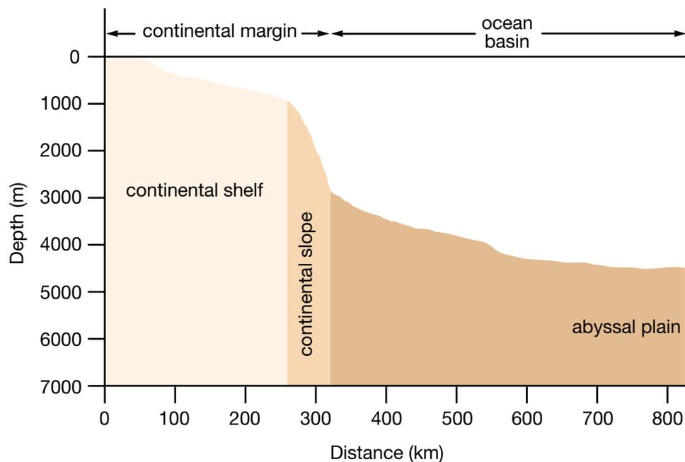
**Figure 5.60** The ocean floor is divided into two main regions — the continental margin (the continental shelf and slope) and the ocean basin.
