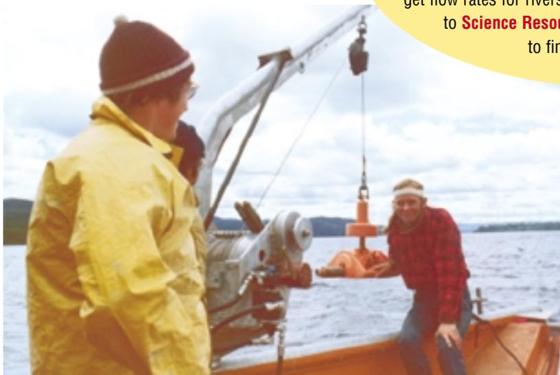
**Figure 5.42** The apparatus shown here “grabs” samples of sediment so scientists can analyze them in a laboratory.
