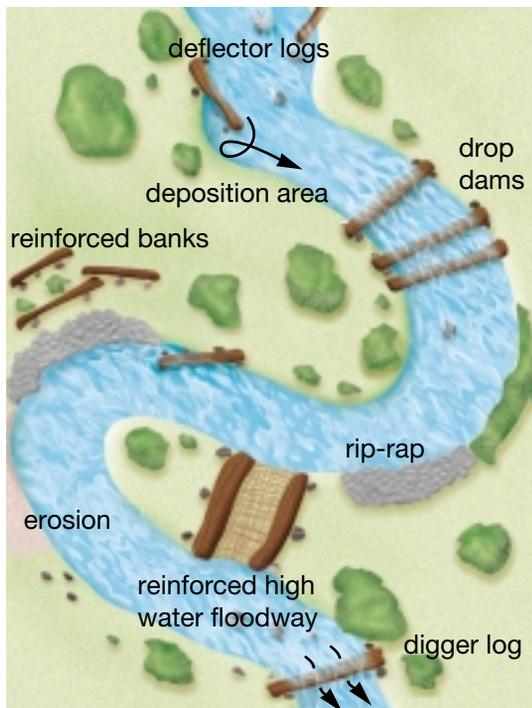
Figure 5.45 Ways of restoring an eroded river
