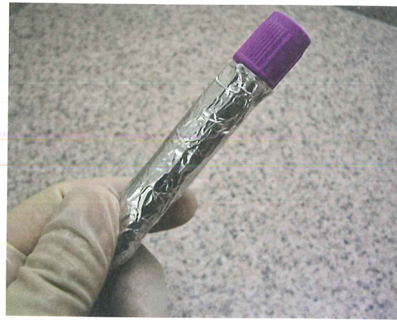
Figure 11-10 Specimens for measurement of substances that are affected by light are usually wrapped in foil.
