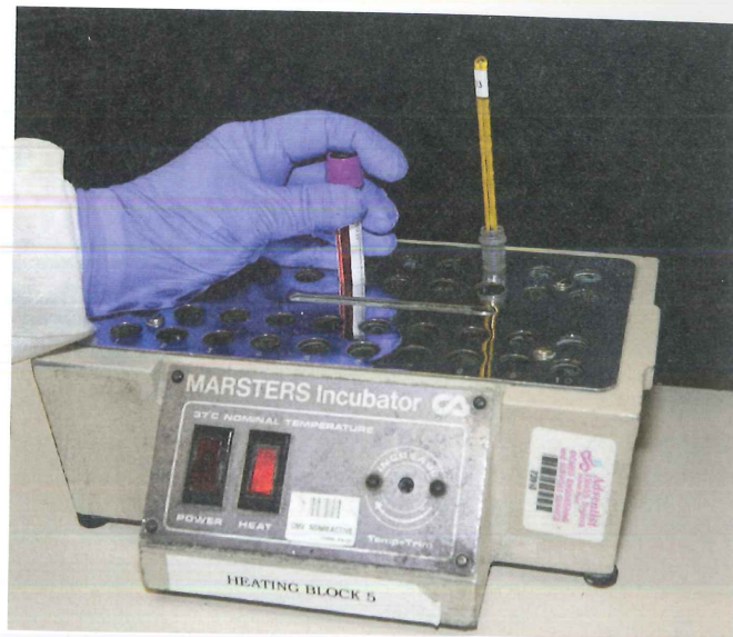
Figure 11-8 Specimens that need to be kept warm can be placed into a heating block set at the correct temperature. Sandra Mesrine/McGraw-Hill Education
