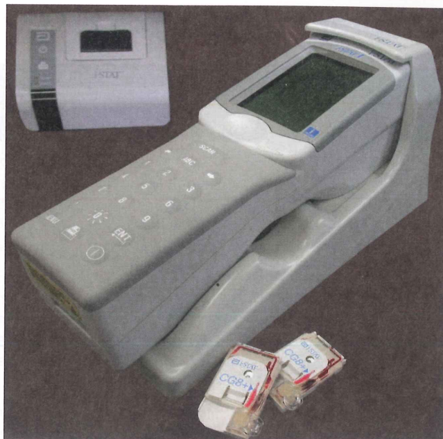
Figure 15-20 Abbott i-STAT ® system: printer, iSTAT analyzer in docking station, and test cartridges. Lillian Mundt
