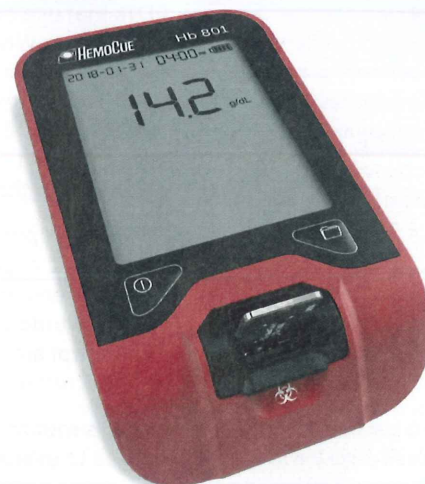
Figure 15-21 HemoCue ® analyzer with microcuvette inserted. Hemocue
