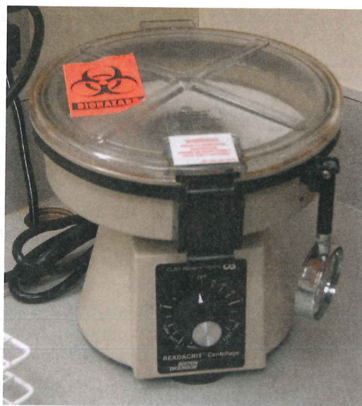
Figure 15-8 Microhematocrit centrifuge. When loading a microhematocrit centrifuge, make sure that the tubes are balanced by placing them directly across from each other, with the sealed ends pointing outward.
