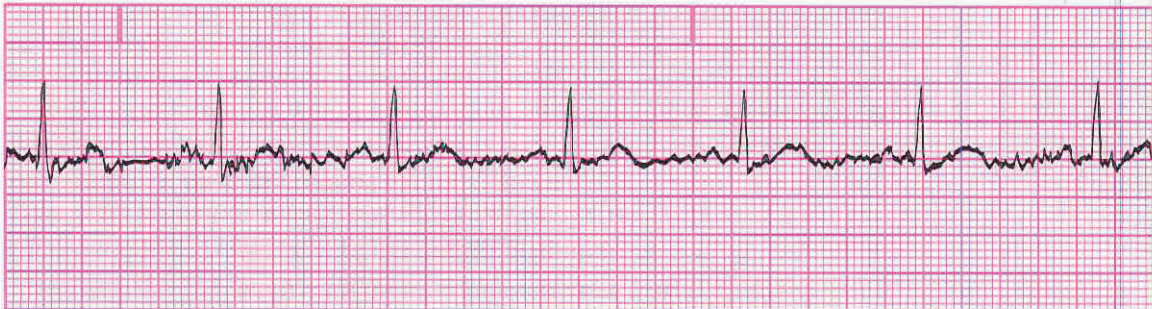
Figure 4-6 Somatic tremor appears as small erratic spikes on the ECG tracing.
