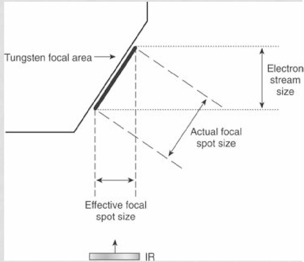
\*The slanted anode angle is called the target angle; can range from 7 to 17 degrees; 12 degrees is the most common
