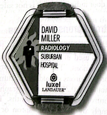
Fig. 11.8 Example of optically stimulated luminescence—type personal dosimeter.
