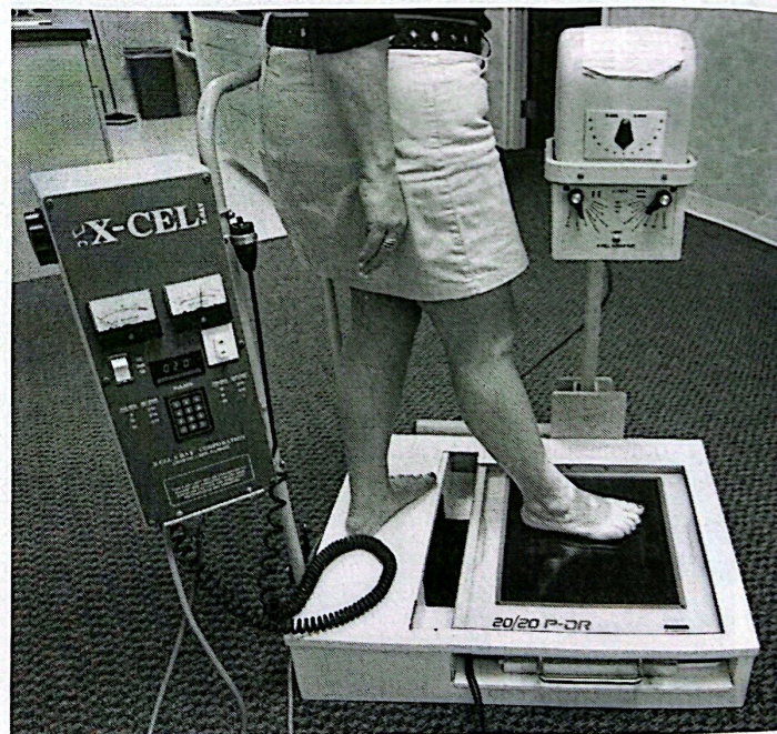
Fig. 2.20 Podiatric x-ray unit designed specifically to image the foot and ankle. This is a self-contained x-ray machine. Note the control console behind the patient and the x-ray tube and collimator above the foot.
