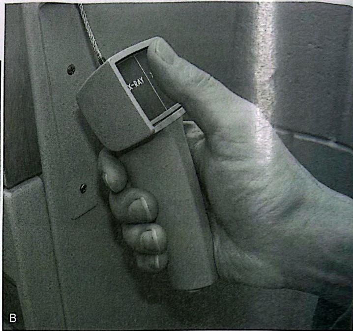
Fig. 6.21 Exposure devices. (A) Two-button finger exposure device. The left finger activates the rotor and, when ready, the right finger initiates the x-ray exposure. (B) Handheld device. The four fingers depress the rotor activator and, when ready, the thumb initiates the x-ray exposure.
