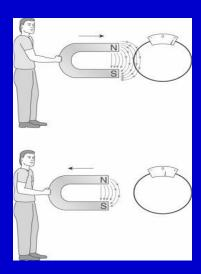
Moving a magnetic field across a conductor also produces AC
