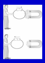
Moving a conductor within a magnetic field will produce an AC
